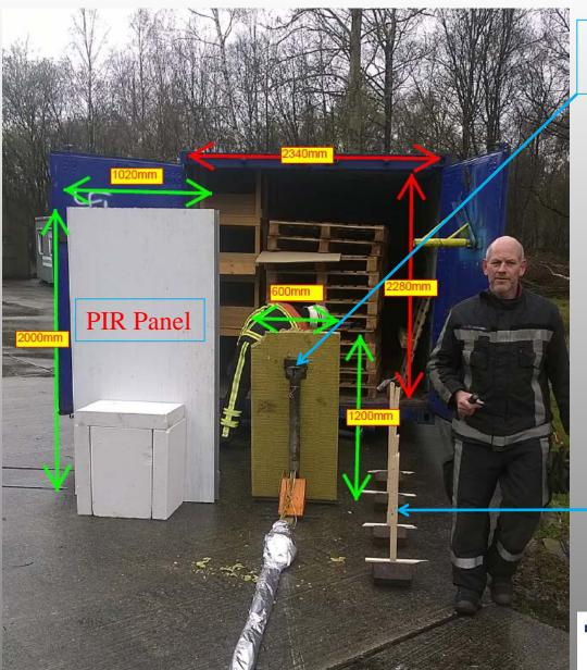
Radiometer (Total Heat Flux type)
