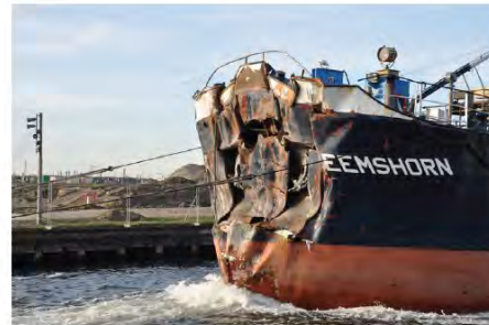
Figure G.6: Deformation of the ship Eemshorn after collision with bridge pier.
