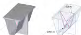
Figure 11.7: A 3D view of the detailed area around a trough to crossbeam connection. A very fine mesh of approximately the thickness of the trough has been used and the rounding at the bottom of the trough is modeled.
