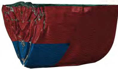
Figure G.5: Deformation of class IV ship during collision process at t=0.27 s.
