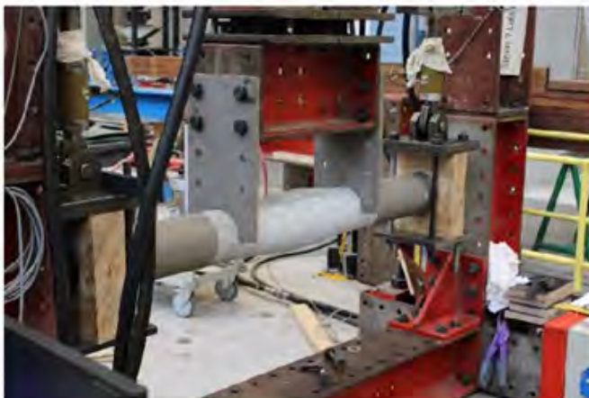
Figure 2 Left: 4-point-bending test set-up in the Stevin laboratory at the Delft University of Technology. On the right the finite element model is shown using symmetry to reduce computational time.
