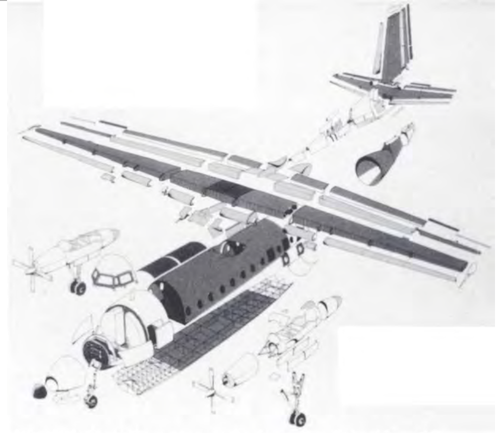
Bonded components in the Fokker Friendship F27 (1950s)
